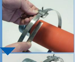
Pull buckle on band, ears pointing towards end of band. Form clamp, holding band on band, then push buckle back over the doubled band, bending the end approx. 1" under buckle.
